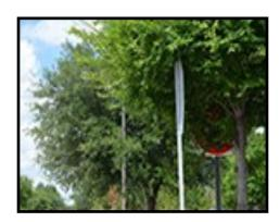
FYI: The pedestrian zone or sidewalk pathway (edge of sidewalk, from the surface to 8 feet above sidewalk), the active transportation zone or multi-use trail pathway (edge of trail, from the surface to 8 feet above trail), and the street or alley corridor (curb line or edge of street or alley, from the surface to 14 feet above street or alley) should be completely clear of overhanging and protruding vegetation.
